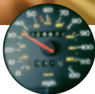
Figure 6 The speedometer in a car measures the car's instantaneous speed. Note the scale markings are given both in km/h and miles per hour, mph.
