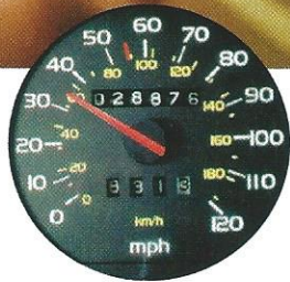
Figure 6 The speedometer in a car measures the car's instantaneous speed. Note the scale markings are given both in km/h and miles per hour, mph.
